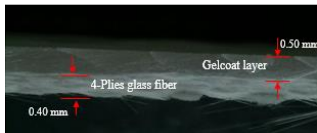
Figure 3. A cross-sectional image of the coated composite.
