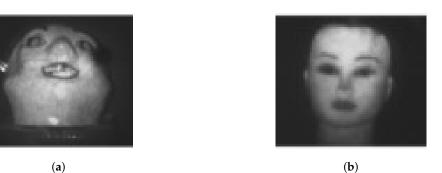
**Figure 5.** Raw image of the test objects captured by the range gated imaging system. (**a**) Raw image of Object 1. (**b**) Raw image of Object 2.
